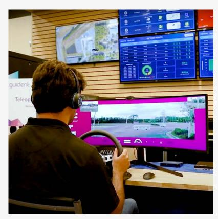
Guident's testbed covers three square miles for developing, testing and validating different use cases that require a fast network with low latency. A reliable network is required to enable a real time monitoring of the autonomous vehicles to ensure safe driving operation and preventing potential accidents before they happen. Guident's Remote Monitoring and Control Center (RMCC) controls the AVs driving performance and collects full road visibility.
